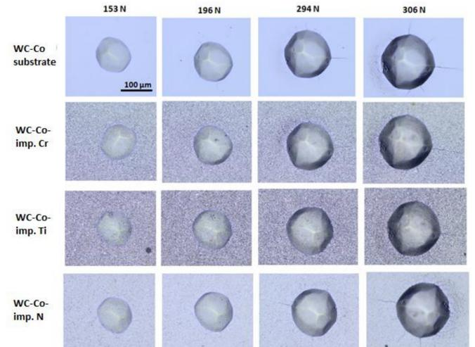
At 294N, cracks appear in the substrate and in the sample implanted with N. At 306N, all samples show cracks, with much less cracks in the samples implanted with chromium and titanium. These results are in agreement with the toughness values obtained.
