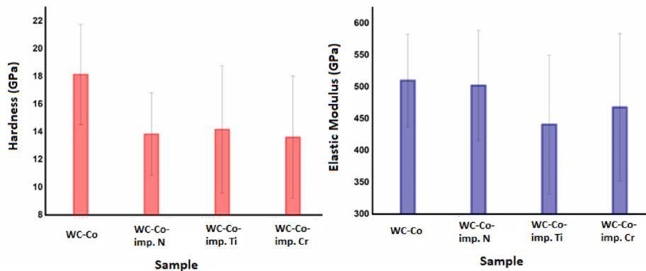
Nanoindentation maps have been made with a Berkovich tip. With a load of 10mN, 30x30 indentations and in a space of 100x100 microns. As can be seen, the implantation of the ions decreases the hardness of the samples. Elastic modulus decreases slightly in the case of chromium and nitrogen, and notably in the case of titanium.
