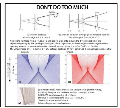
We have used two software packages: CPO (electronoptics.com, boundary element method) and COMSOL (www.comsol.com, finite element method).
